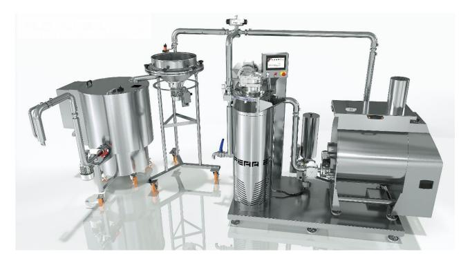
Fully automatic mixing, conching and refining line designed for small and medium-sized productions.
